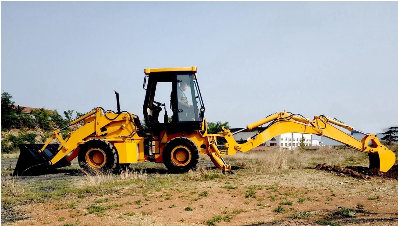
**Loader bucket capacity 1.2cbm/ 2500kg, Digger bucket capacity 0.3cbm**
