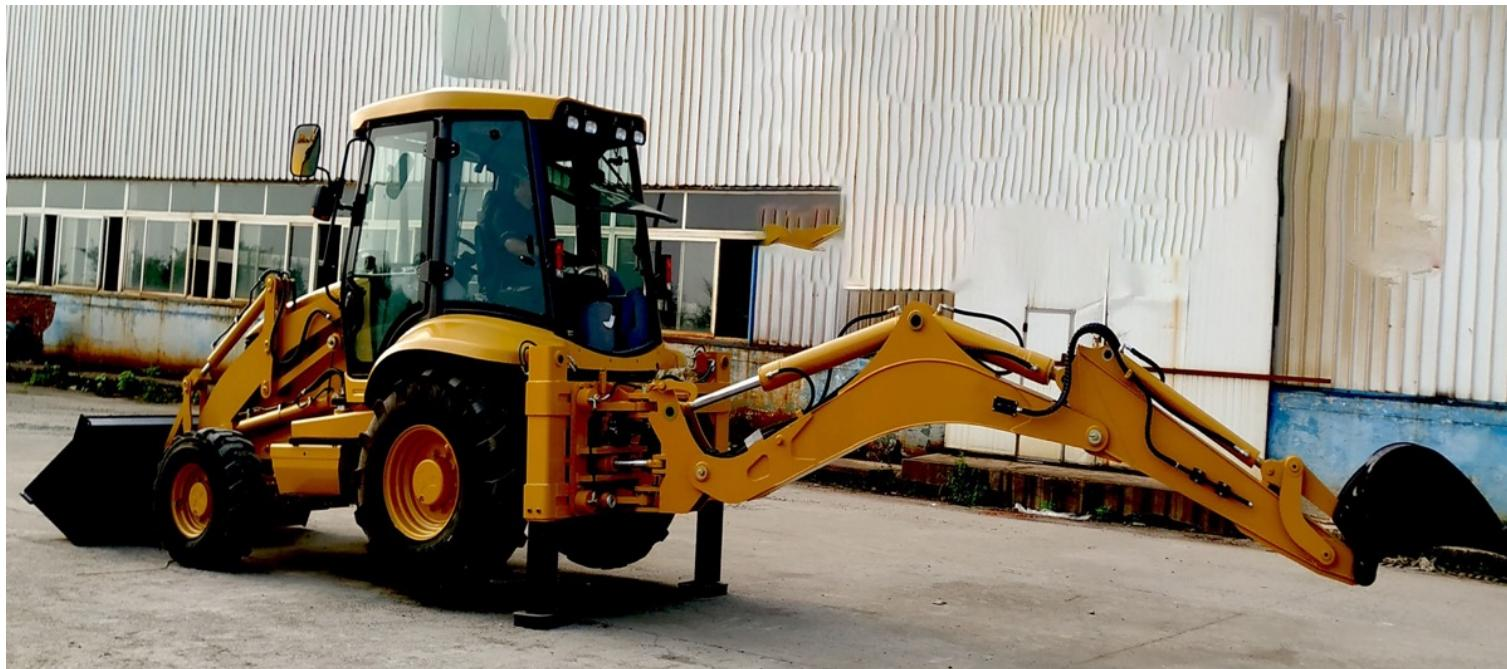
Loader bucket capacity **1.0cbm/ 2500kg**, Digger bucket capacity **0.3cbm**
