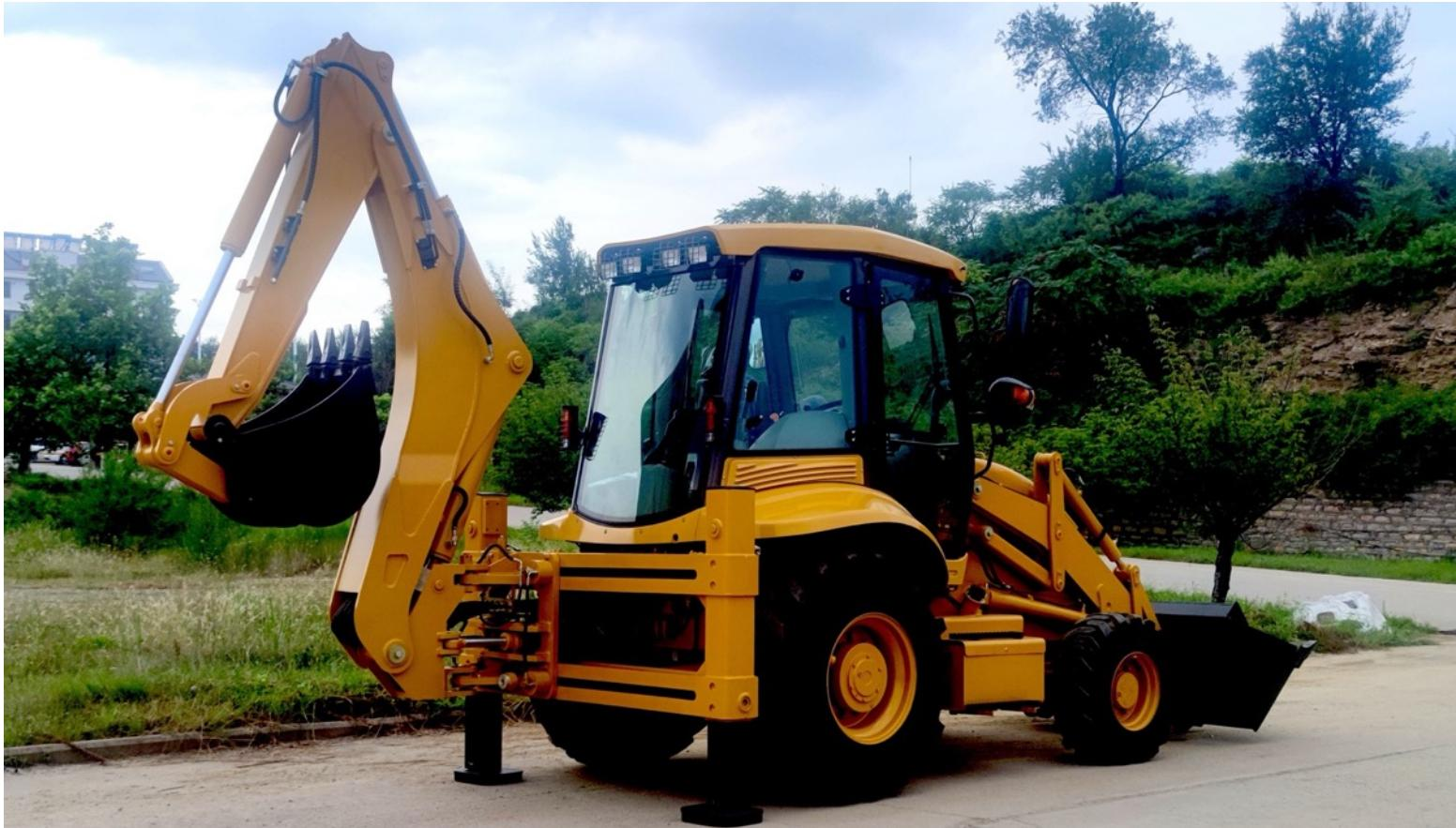
Loader bucket capacity **1.0cbm/ 2500kg**, Digger bucket capacity **0.3cbm**
